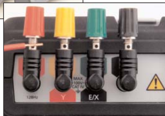
Terminal Adapters are optional accessories used to allow the DET3 and DET4 Series units' terminals to accept alternative cable connections.
